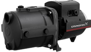
JPA is a self-priming, single-stage centrifugal pump with a body made of cast iron. It has an axial suction port and radial discharge port. The pump has a built-in ejector with guide vanes for optimum self-priming properties.
